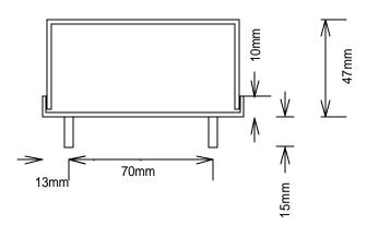
Fixings - 2 off M4 studs fitted to base of unit (marked 'A').
